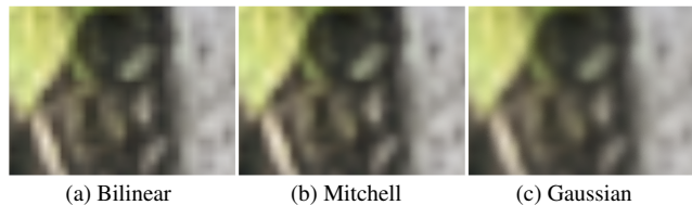
Figure 6: Bilinear filtering (a) compared to stochastic, single sample estimation of the bicubic Mitchell (b) and Gaussian (c) filters, resolved with DLSS’s temporal accumulation. The bicubic Mitchell filter is much sharper than the bilinear filter and does not produce diamond-like artifacts. The Gaussian filter is isotropic and although it tends to blur textures, it produces the most pleasing and natural reconstruction of diagonal lines.
