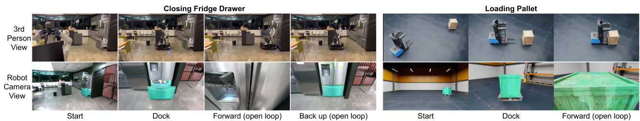
Fig. 11. Using AMR for mobile manipulation tasks. Left: closing a fridge drawer by pushing the robot body towards the drawer. Right: forklift loading a pallet. AMR accurately tracks the target objects throughout.
