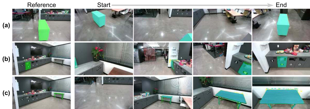
Fig. 10. Real-world qualitative experiments in new scenes. Left: reference image with target object highlighted by the green mask. Remaining columns: robot's camera view while moving. The tracked object is highlighted by the cyan mask. The tasks are: (a) Go to the back of the cabinet and stand 0.8 m away. (b) Go to the front of the landfill trashcan and stand 1 m away. (c) Go to the front of the table and stand 0.5 m away.
