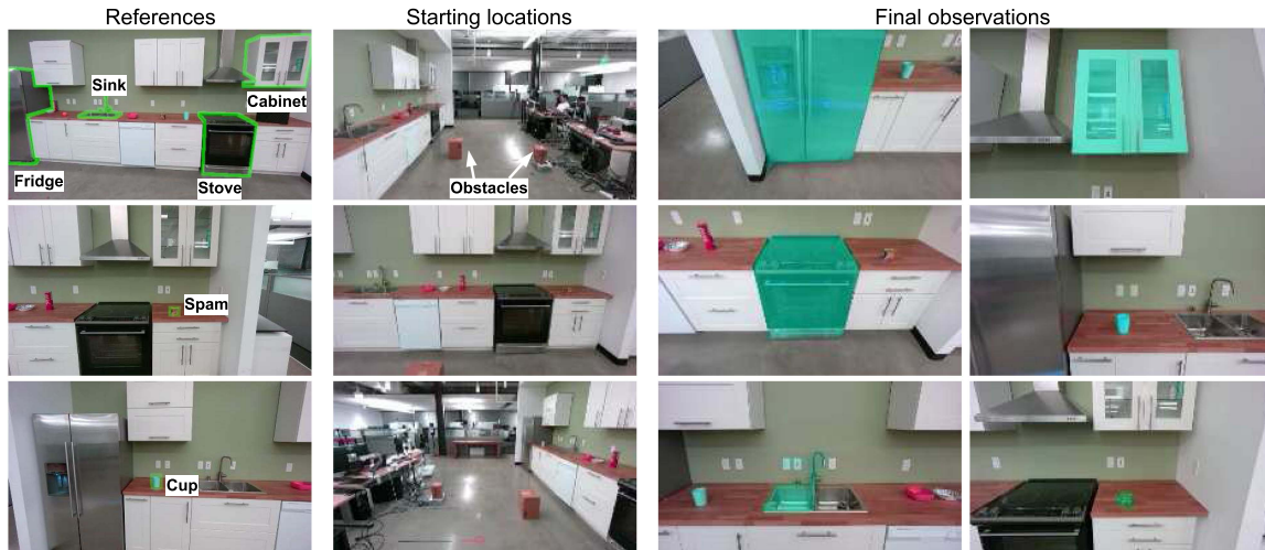
Fig. 9. Real kitchen experiments. Left: reference images and contours of target object masks. While the fridge is partially out of view, the model can still reach the fridge. Middle: Initial view of the scene through the tilt camera. Right: robot observations after reaching each object overlaid with predicted masks (in cyan).
