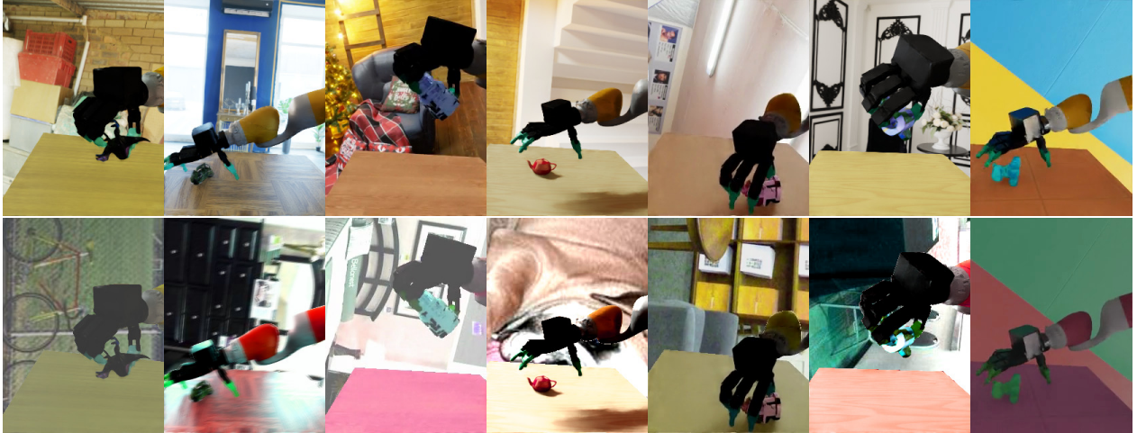
Figure 20: Top: Camera renderings from different environment instances in simulation, adapted from Singh et al. (2025) . Bottom: Examples of data augmentations applied to these renderings before passing them to the learning agent.
