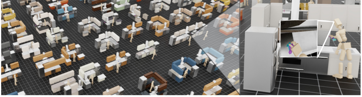
Figure 29: Perceptive Dexterous Control (PDC) (Luo et al., 2025) enables a humanoid equipped with egocentric vision to search, reach, grasp, and manipulate objects in cluttered kitchen scenes. PDC uses visual perception as the sole indicator of which hand to use, which object to grasp, where to move, and which drawer to open.
