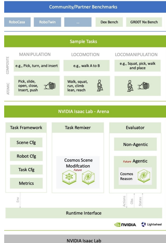
Figure 34: The architecture diagram of Isaac Lab - Arena , a framework and collaborative ecosystem for accessible and scalable policy evaluation in simulation.
