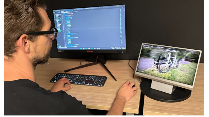
Fig. 11. Real-time interactive 3D radiance field demonstration on a Looking Glass light field display, enabling users to dynamically change viewpoints and visualize radiance fields in a 3D space (see supplementary video).
