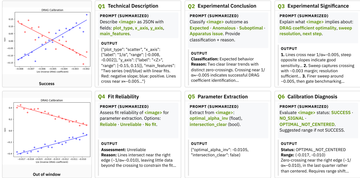
Figure 3 | The six question types in QCalEval, illustrated on a DRAG calibration example. Q1 uses a universal prompt across all families; Q2–Q6 prompts are customized per experiment family with family-specific background context, failure mode definitions, and parameter extraction schemas.
