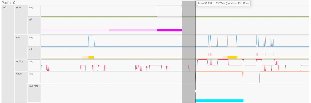
Fig. 14. This view is further expanded to highlight the handoff from the last application GPU task (shown in magenta) to the first checkpoint copy from GPU framebuffer to zero-copy memory (shown in teal). Lightly shaded boxes represent tasks that are blocked, medium-shaded portions represent tasks that are ready but not yet executing, and brightly-colored boxes represent running tasks. The small, pink boxes on the CPU are Legion internal meta-tasks used to collect profiling data, and would not appear in a production run of this application.
