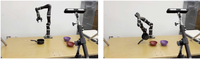
Grasp slippage caused a motion planning failure.
