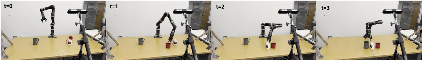
Fig. 1: Real-world rearrangement with unseen objects, given a language instruction. We use StructDiffusion to predict possible goals that satisfy physical constraints such as avoiding collisions between objects. At the core of StructDiffusion is an object-centric multimodal transformer backbone combined with a diffusion model, capable of sampling diverse high-level motion goals for language-guided rearrangement.
