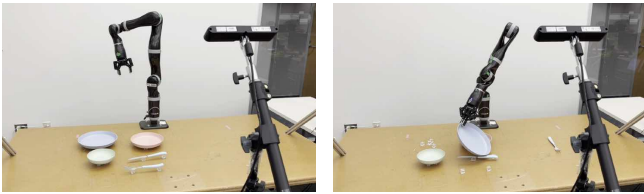
The planned motion failed to avoid another object.
