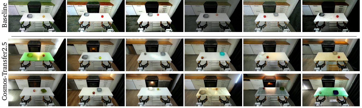
Figure 11: Real-Robot Data Augmentation Gallery. We show the baseline (top row) and [Cosmos-Transfer2.5-2B] (bottom two rows) data augmentation samples.
