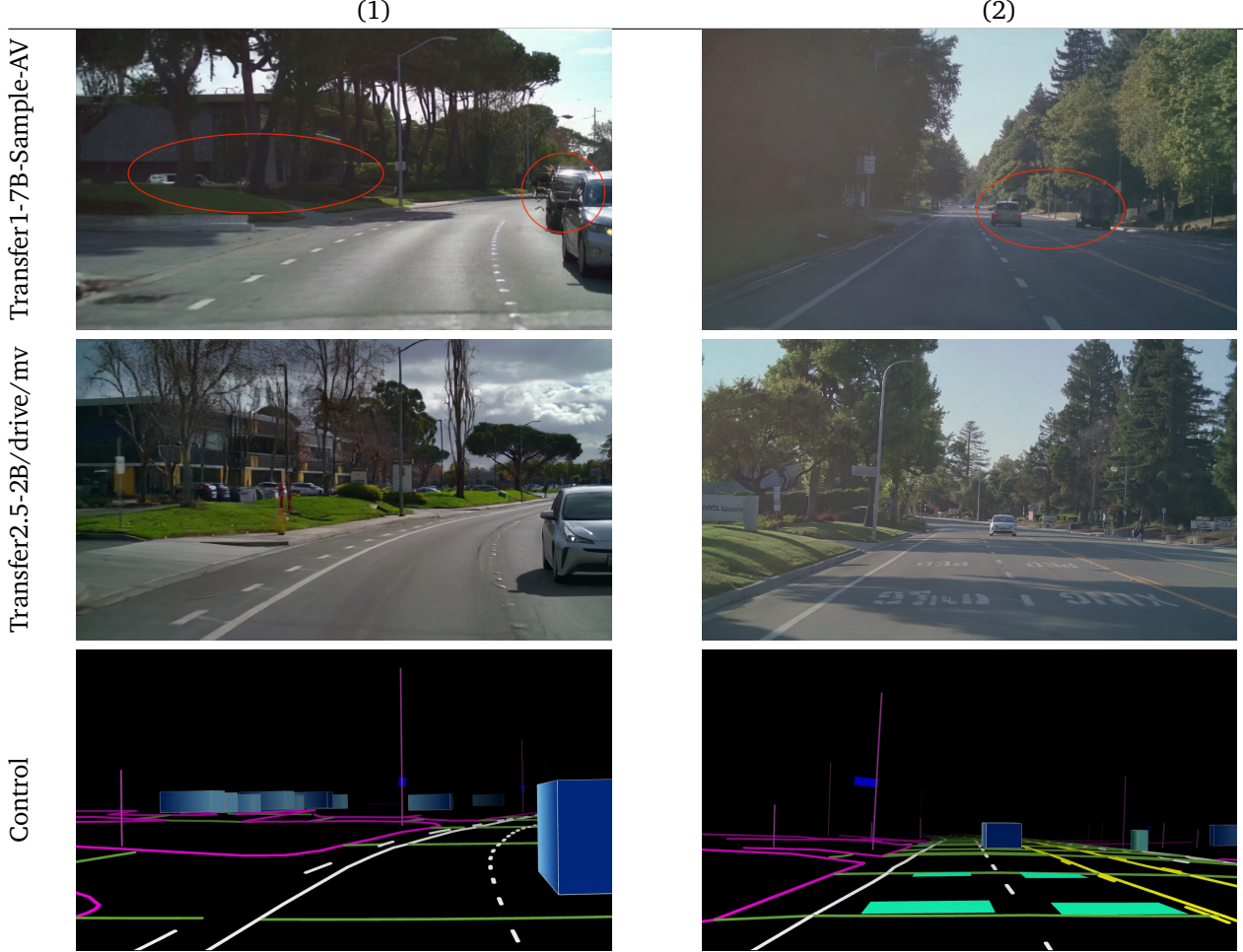
Figure 14: Comparative controlled generations between [Cosmos-Transfer1-7B-Sample-AV] and [Cosmos-Transfer2.5-2B/auto/multiview]. In example (1), we can observe that [Cosmos-Transfer1-7B-Sample-AV] hallucinates a distorted black car behind the silver vehicle, which is described neither in the text prompt nor in the control video. We can also observe the lack of alignment to the control signal when generating the parked vehicles behind the grassy mounds. In example (2), we can observe that [Cosmos-Transfer1-7B-Sample-AV] renders the vehicle in the central lane driving on the wrong side of the street with an incorrect orientation, as well as a truck instead of a pedestrian close to the sidewalk. All these inconsistencies are resolved in [Cosmos-Transfer2.5-2B/auto/multiview].
