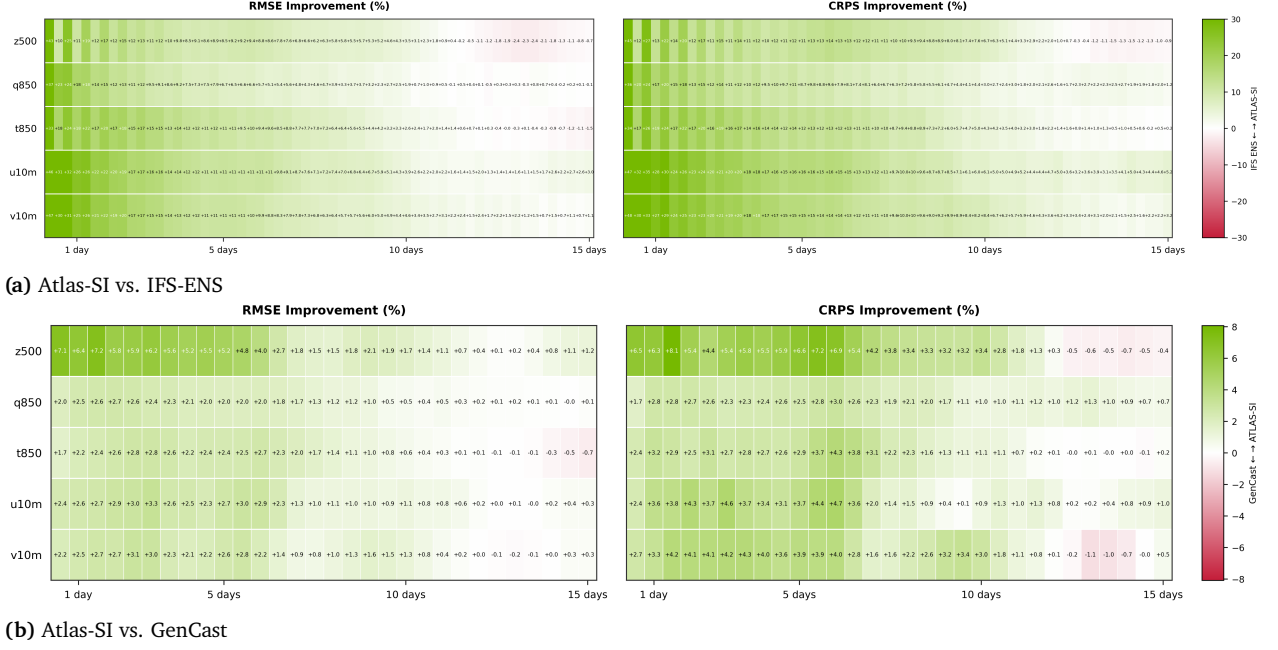
Figure 1: Scorecard comparison of ATLAS-SI vs. IFS-ENS (a) and GenCast (b) for a fifteen day forecast with 56 ensemble members averaged over ERA5 initial conditions in 2020. Left shows percent improvement in the RMSE of the ensemble mean and right in the ensemble CRPS.
