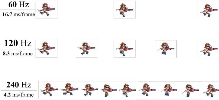
Fig. 1. Visual smoothness and frame rate. Each row shows the same avatar movement rendered at a different frame rate (60, 120, and 240 Hz). At higher frame rates, more frames are presented per second, so each frame captures a smaller change in the avatar’s animation and position, and motion appears smoother to the player.
